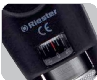
The slit image can be turned 360° with the knurled thumb screw. The respective angle read-out is displayed directly on the scale.
