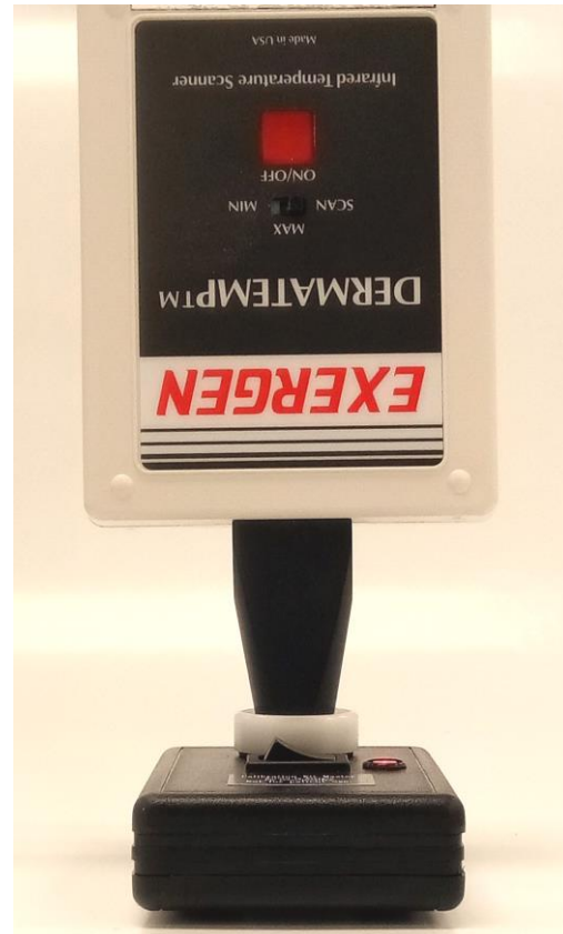
Figure 1. Portable black body is used to verify the calibration of any DermaTemp model vs. a Certified Master, by comparison of readings.
