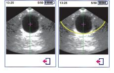
**Bladderpoint™** is a proprietary bladder targeting system used in Pre-scan mode to get a quick and accurate scan by placing crosshairs on the fluid in the bladder.
