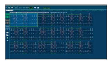
Rapidly view and edit events and add the most severe events to the summary report. The full-disclosure ECG can be rapidly and clearly viewed to verify the analysis, clean up areas of artifact, and identify events. Scroll and zoom functions are available on a single display or on a synchronized second display.
